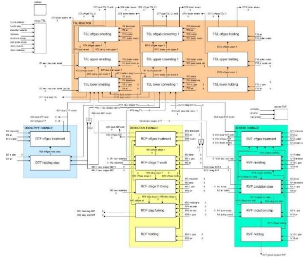
Figure 1 – Modelling of the entire secondary copper production route with a smelting reactor, a converting step, and a refining step including a drum type furnace as a mixing and holding aggregate [1]
