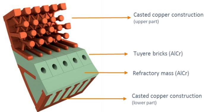
Figure 9 – Advanced CFM (composite furnace module) cooler for cooling tuyeres of a Peirce Smith converter
