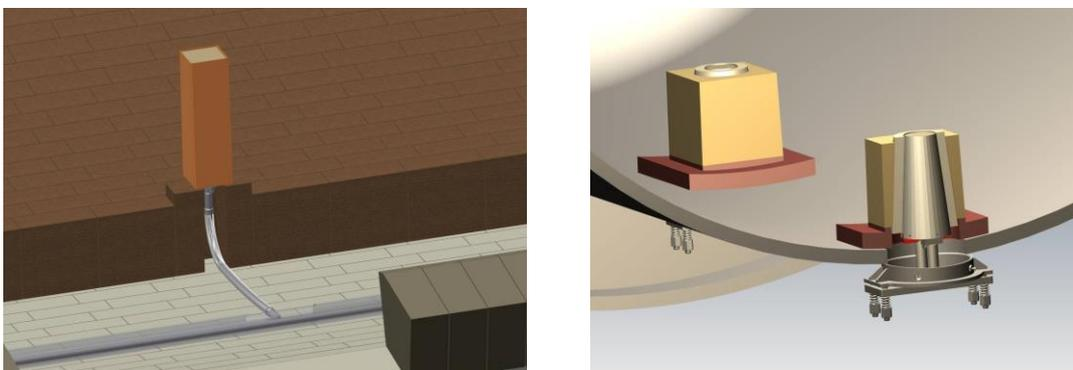
Figure 3 – Different systems of purging plugs available, non-changeable system with internal piping (left) and changeable system with external piping (right) [3]
