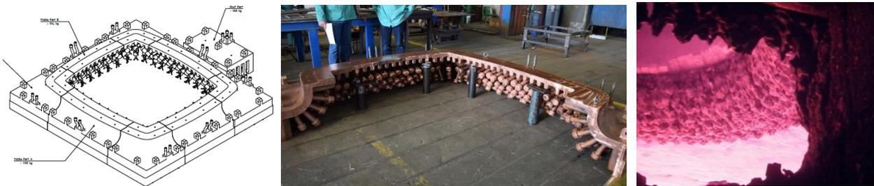
Figure 7 – CFM (composite furnace module) cooling element for charging mouth of an anode furnace
