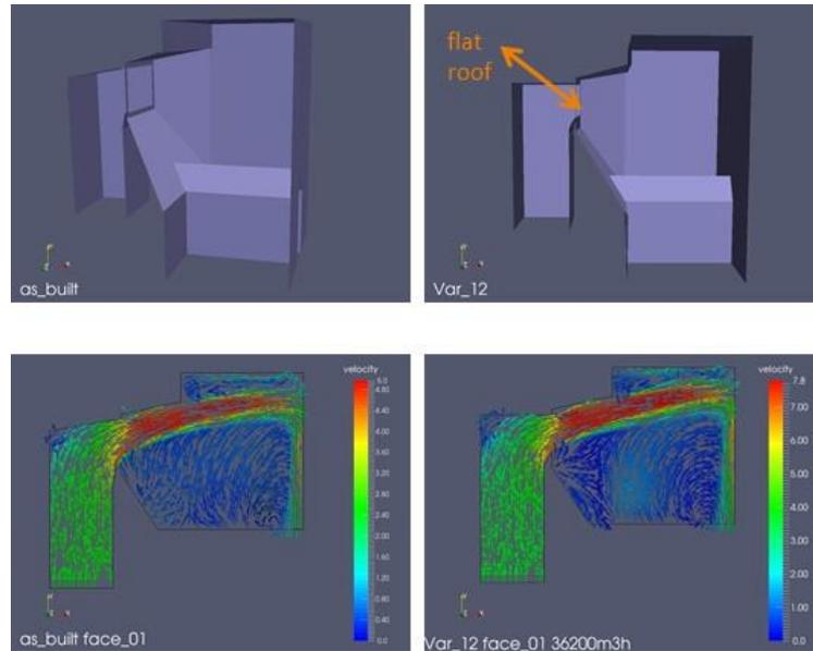
Figure 5 – Vanyukov-furnace post-combustion chamber; Flow model for optimized geometry of the post-combustion chamber for preventing any built-ups as a result of preferably high offgas velocity
