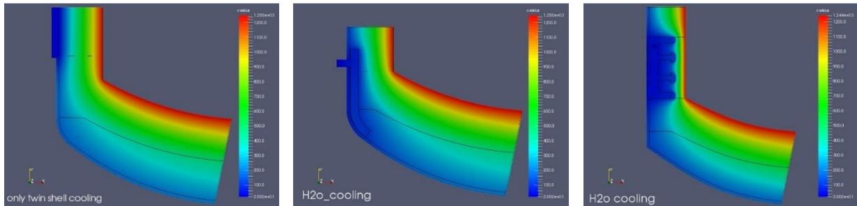
Figure 6 – CFD Model of the temperature distribution depending on different cooling solutions for the cooling of a furnace side wall, cooled plate at the outside of the steel shell (left), inside the steel shell (middle) and high intensity cooler (right)
