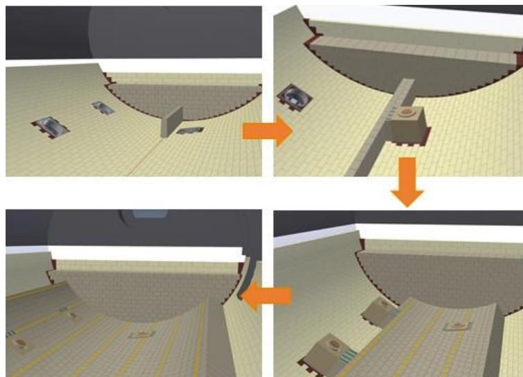
Figure 4 – Example of a 3D model of the entire refractory lining of an anode furnace: single steps for the step by step lining sequence including purging plugs
