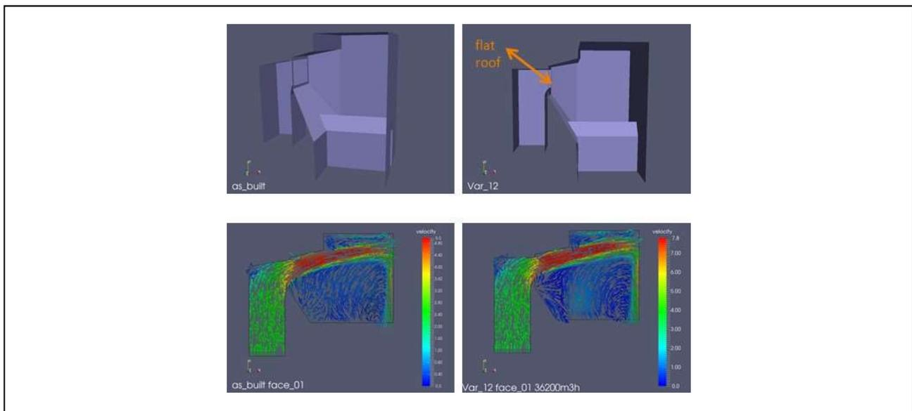
Figure 2: Vanyukov-furnace post-combustion chamber; Flow model for optimized geometry of the post-combustion chamber for preventing any built-ups as a result of preferably high off-gas velocity
