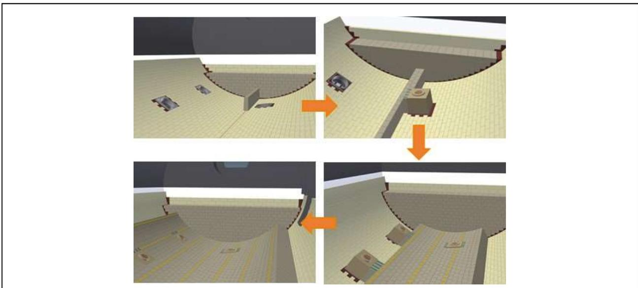
Figure 4: Example of a 3D model of the entire refractory lining of an anode furnace: single steps for the step by step lining sequence including purging plugs
