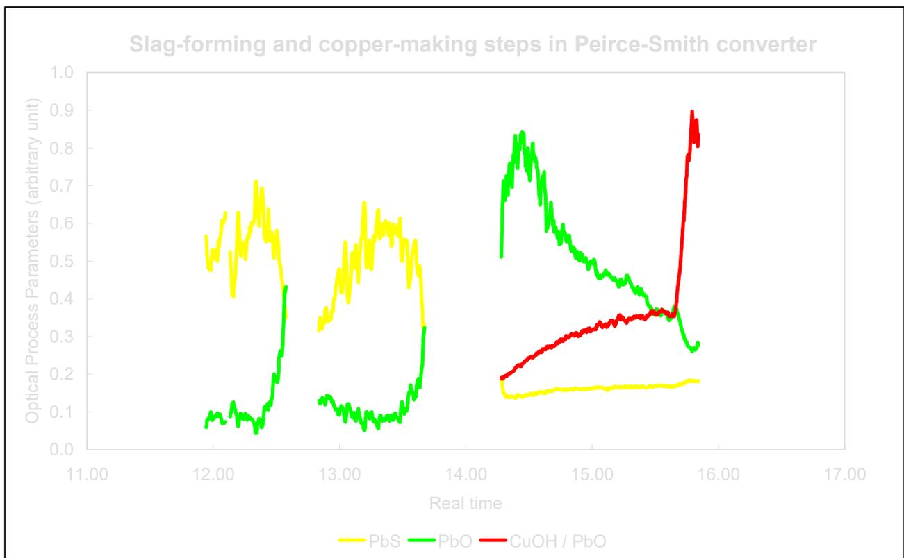
Figure 3: Online process parameter reading during a Peirce Smith converter cycle; OPC system SEMTECH, Wilhelm Wendt
