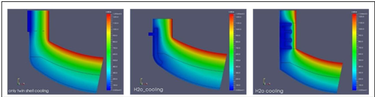
Figure 5: CFD Model of the temperature distribution depending on different cooling solutions for the cooling of a furnace side wall, cooled plate at the outside of the steel shell (left), inside the steel shell (middle) and high intensity cooler (right)
