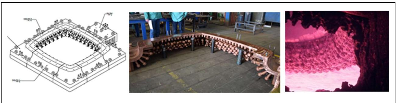
Figure 6: CFM cooling element for charging mouth of an anode furnace
