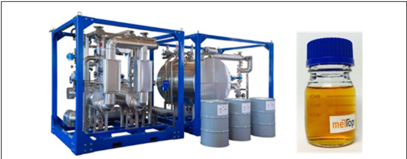
Figure 7: Basic design of an ILTEC system as installed at ArcelorMittal Bremen GmbH in Germany (left) and photo of the optical appearance of the ionic liquid IL-B2001
