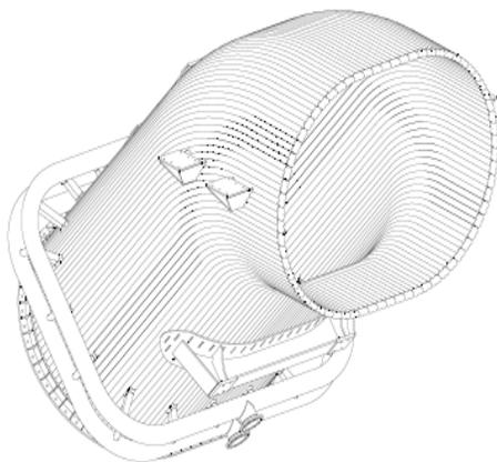
Figure 7 – Water cooled part of the offgas duct of an EAF
