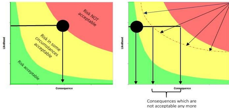
Figure 4 – 2-dimensional risk analysis of a state of the art water cooled area (left) and using the ionic liquid as cooling medium (right) [5]
