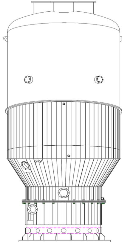
Figure 8 – Construction drawing of the shaft furnace where cooling of the lower part of the shaft is realized with ILTEC Technology
