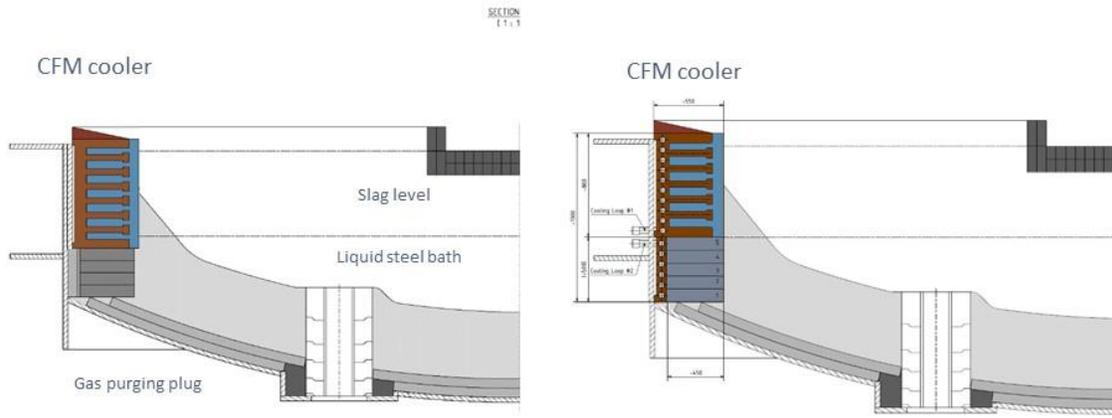
Figure 6 – Different opportunities for installation of a high intensity cooler within the side wall of an EAF, left: installation of the cooler only at the slag line; right: slag line cooling with CFM elements and cooled copper plate behind the brick lining at the lower part
