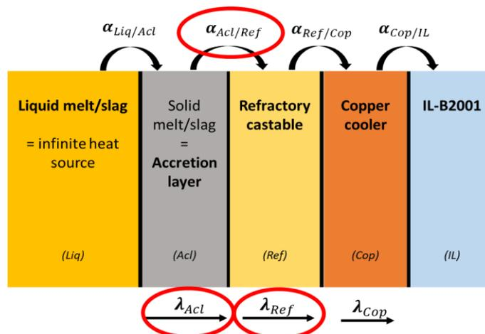
Figure 1 – Schematic picture of the different layers within the entire system in industrial scale use within a copper cooling element
