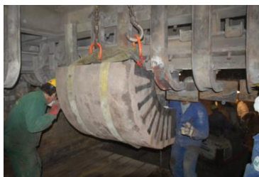
Figure 9 – Off-gas junction of an anode furnace
