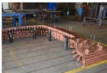
Figure 8 – Off-gas opening for an electric arc furnace
