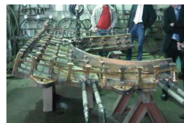
Figure 10 – Charging mouth of a tilting furnace
