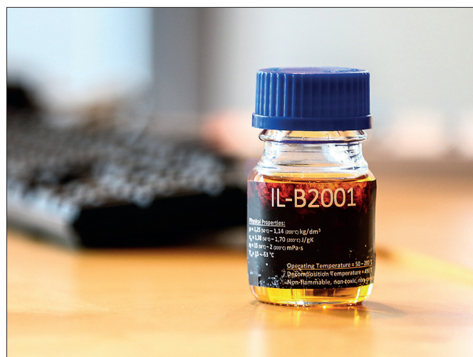
Fig. 5: Water-free cooling solution – ionic liquid IL-B2001 (source: Met-top GmbH)
