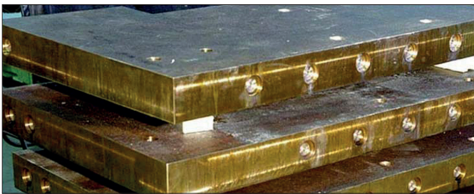
Fig. 3: Drilled copper coolers
